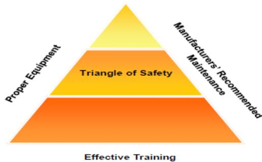
The successful use of any type of fire equipment - fire extinguishers, fire suppression systems, hose lines, nozzles or even apparatus - depends upon three elements being in place at the same time: Equipment – Maintenance – Training.
